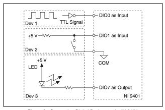
Figure 3. Connecting Digital Devices to the NI 9401
